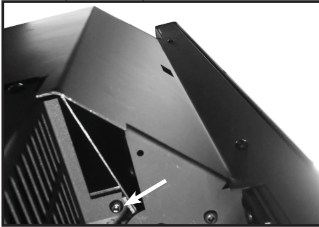
13. Screw the fan assembly to the appliance: 2 screws (1 each side) into the firebox bottom.
