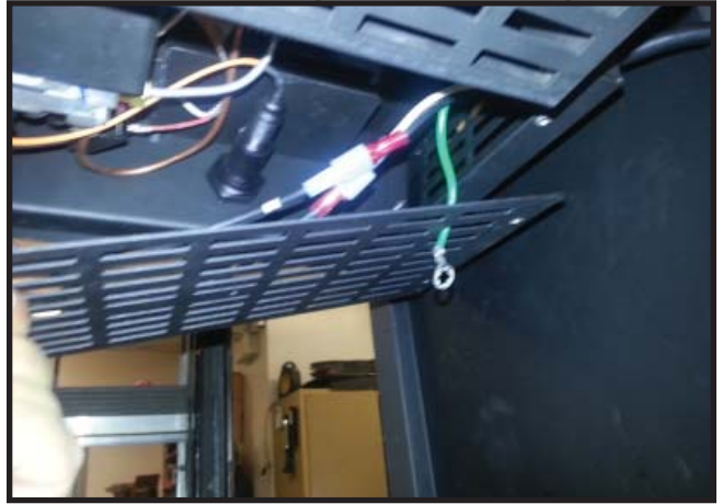
Screw the power cord ground wire to the wire cover and control housing side.
