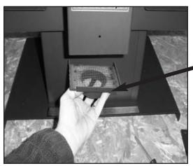
Remove the main air tube adapter from the packaging. Slide the adapter onto the bottom of the main air tube.
