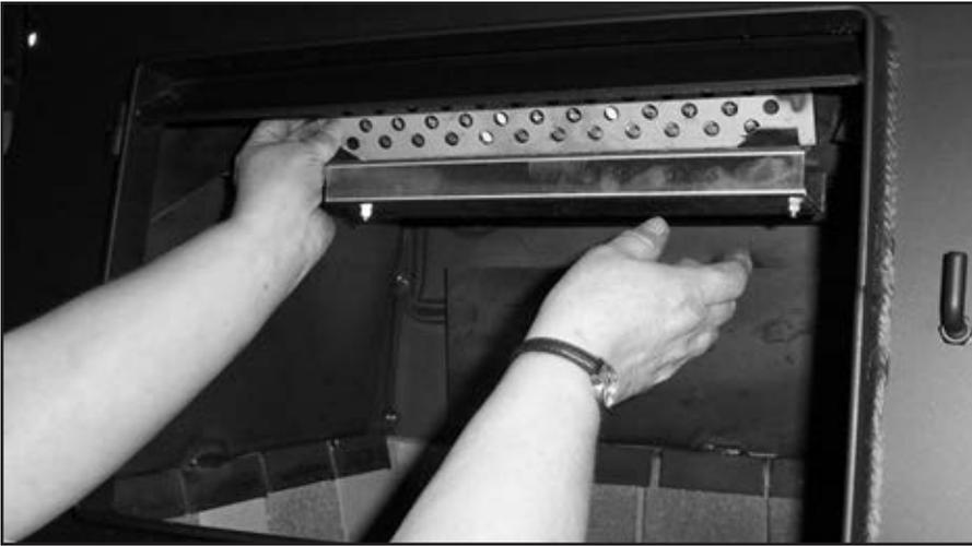
Remove the flame shield from the stainless retainer clips. This can be done through the front loading door. Pay particular attention to the direction the flame shield was installed as there is a correct way to install the unit. The side triangles must point towards the rear of the stove. No tools are required for this process.
