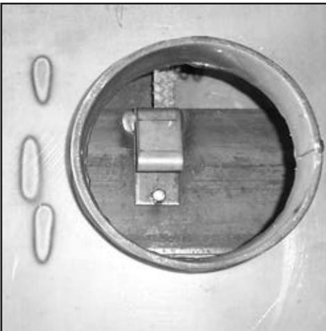
To remove the bypass plate, the plate must be in the position as shown to the left. This can be achieved by moving the bypass rod out of the way and lift one end of the bypass plate for clearance to turn inside the top assembly. Once the bypass plate is in this position, remove the plate through the combustor area. For purposes of clarity, the picture to the left is of the top assembly.
