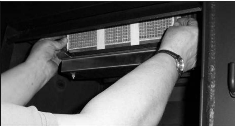
Remove the catalyst very carefully. The best method is to use two small flat head screw drivers and gently pry the combustor forward. Make certain the blade of the screwdrivers are between the stainless steel band and the stove housing. Once pried forward 1/4", then grip each side of the combustor and gently remove. Set the combustor to the side in a safe place.
